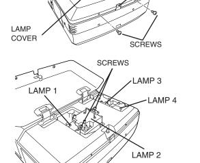
Make sure which number of lamp needs to be replaced on Lamp Status Display. Figure shows case of replacing LAMP 2.
